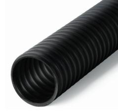
A versatile solution for suction and light blowing of lightweight abrasives. Its SBR rubber blend with static carbon black ensures exceptional abrasion resistance and static dissipation. Ideal for materials like rockwool, fiberglass, sawdust, grain, insulation, and cement dust.
