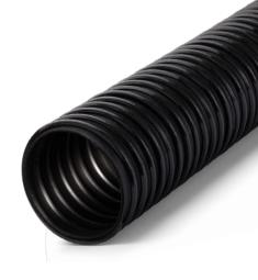
A versatile solution rated to 220°F. Combining abrasion resistance with flexibility, it's ideal for lightweight abrasives like sawdust, grass clippings, street refuse, and cotton pickers. Constructed with EPDM rubber, a metal wire helix, a smooth bore, and a slightly corrugated outer diameter.
