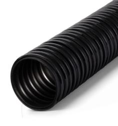
A versatile solution with a wear strip for light dragging. Combining abrasion resistance with flexibility, it's ideal for lightweight abrasives like sawdust, grass clippings, street refuse, and cotton pickers. Constructed with EPDM rubber, a metal wire helix, a smooth bore, and a slightly corrugated outer diameter.
