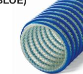
A versatile solution for combined vacuum, higher working pressures, and increased flexibility. Lightweight and flexible with an external helix for easy drag, it's ideal for colder environments and liquid fertilizer applications. Constructed with flexible cold weather PVC, a rigid PVC helix, synthetic braiding, smooth bore, and corrugated outer diameter, it ensures reliable performance and visual material flow checks.
